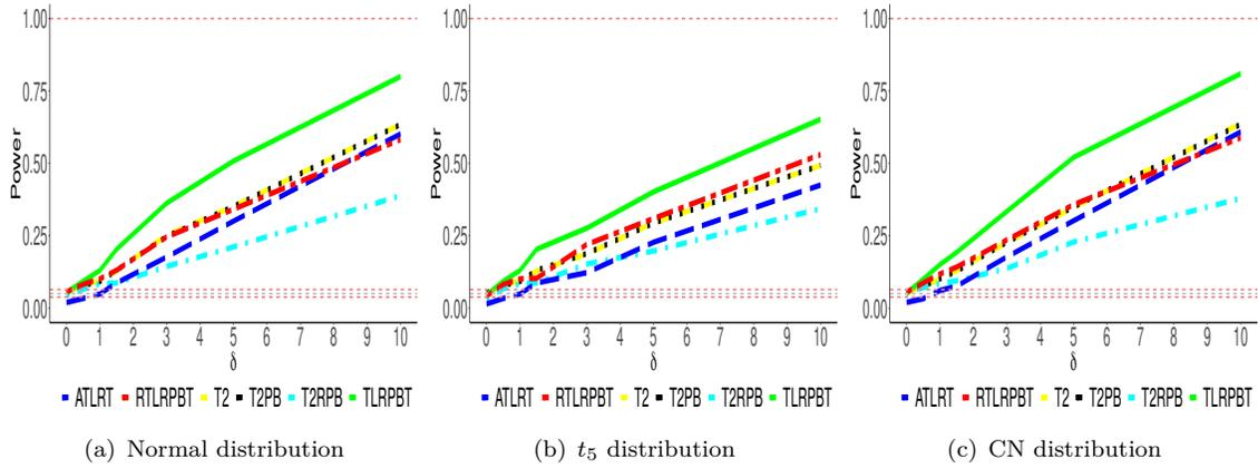
Figure 1. Power of the tests as a function of the generalized Mahalanobis distance  $\delta$  between the parametric and hypothetical vector means, with  $n = 10$  and  $p = 2$ , where the gray lines represent the lower and upper limits of the exact binomial interval and the maximum power.
